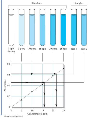
Figure 1F-2 Constructing and using a calibration curve to determine the concentration of arsenic. The absorbance values are plotted against the concentrations of the solutions in the cuvettesFinally, the concentrations of the unknown solutions are read from the plot, as shown by the dark arrows.
