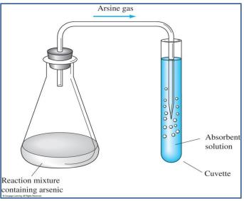
Arsine bubbled into the solution in the cuvette reacts with silver diethyldithiocarbamate to form a colored complex compound according to the equation:
